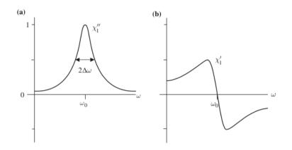
Figure 2: Susceptibility of the two level system. Figure taken from (gry)
