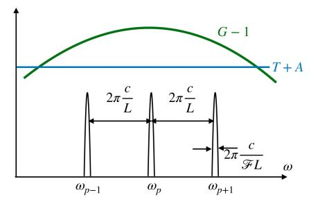
Figure 4: Frequency distribution of the steady-state laser.
