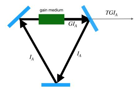
Figure 1: The Laser set-up.
