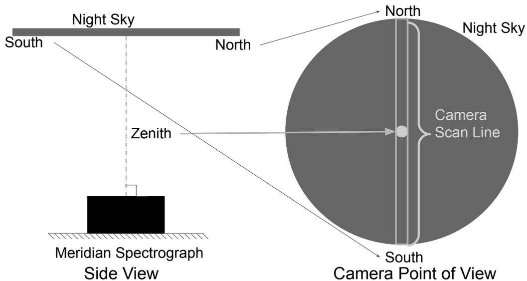
**Figure 1.** Schematic of keogram imaging system. The left shows a side view of a meridian spectrograph looking up local zenith and the right shows a view of the night sky from the perspective of a camera as the meridian spectrograph takes a one-pixel-wide scan from horizon to horizon through local zenith.
