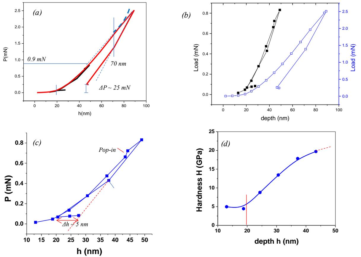
Fig 1 (a) Load-depth (P-h) plot for nanoindentation on TiB<sub>2</sub>/Si coatings (a) in same load axis for two different depths (b) separate load axis (c) individual lower depth and (d) corresponding hardness.
