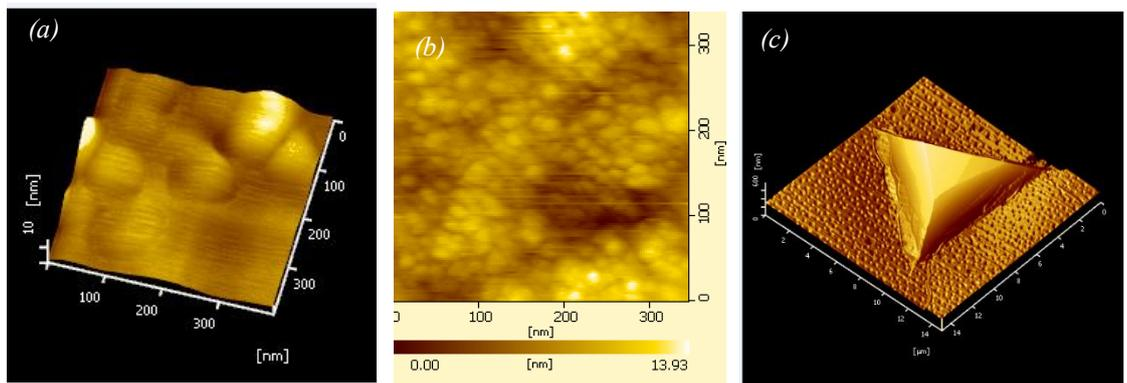
Fig 2. The surface of TiB<sub>2</sub> coating with formation of (a) large grains having (b) clustering of nanocrystallites and (c) pile-up (swelling) occurring during nanoindentation.
