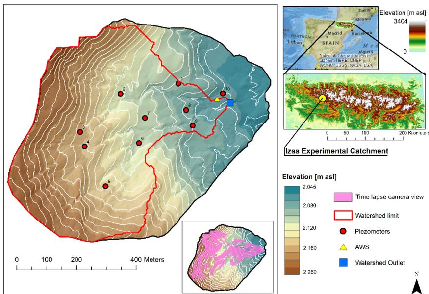
**FIGURE 1.** Izas catchment and the location of the automatic weather stations (yellow triangle) and gauging stations (blue square) and piezometers (red circles). Red line outlines the drainage area of the gauging station. Pink areas in the small map indicates the surface covered by the time lapse camera.
