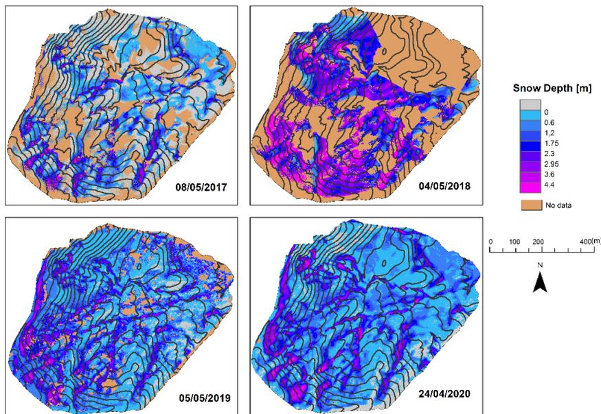
**FIGURE 3.** Snow depth for different dates with available data closer to the annual maximum snow accumulation. Snow depth records are acquired by using a TLS (2017 and 2018) and a UAV (2019 and 2020).
