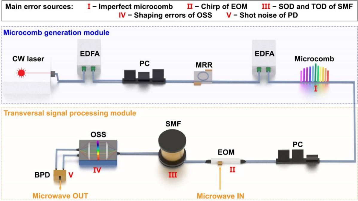
**Fig. 2.** Schematic of a practical microcomb-based MWP transversal signal processor. The main error sources are labelled as I – V. CW laser: continuous-wave laser. EDFA: erbium-doped fibre amplifier. PC: polarization controller. MRR: microring resonator. EOM: electro-optic modulator. SMF: single-mode fibre. OSS: optical spectral shaper. BPD: balanced photodetector. SOD: second-order dispersion. TOD: third-order dispersion.
