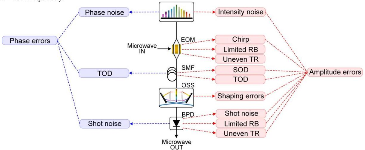
**Fig. 10.** Amplitude and phase errors induced by different components in microcomb-based MWP transversal signal processors. EOM: electro-optic modulator. SMF: single-mode fibre. OSS: optical spectral shaper. BPD: balanced photodetector. RB: response bandwidth. TR: transmission response. SOD: second-order dispersion. TOD: third-order dispersion.
