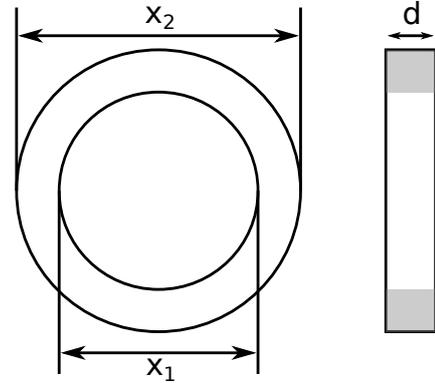
**Figure 4:** Dimensions of borosilicate glass and spacers for phantom samples with  $x_1 = 18$  mm,  $x_2 = 25$  mm and  $d = 0.1$  mm,  $d = 0.2$  mm,  $d = 0.3$  mm or  $d = 0.5$  mm.
