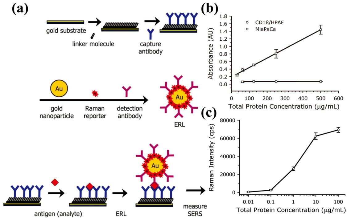
**Figure 6.** (a) Schematic of SERS-based immunoassay for MUC4 and CA19-9; (b) ELISA measurements of CD18/HPAF (positive control) and MiaPaCa (negative control) lysates; (c) Dose-response SERS curve for CD18/HPAF in PBS buffer. Adapted and reproduced from ref. 75 with permission from the American Chemical Society (ACS) Copyright 2011.
