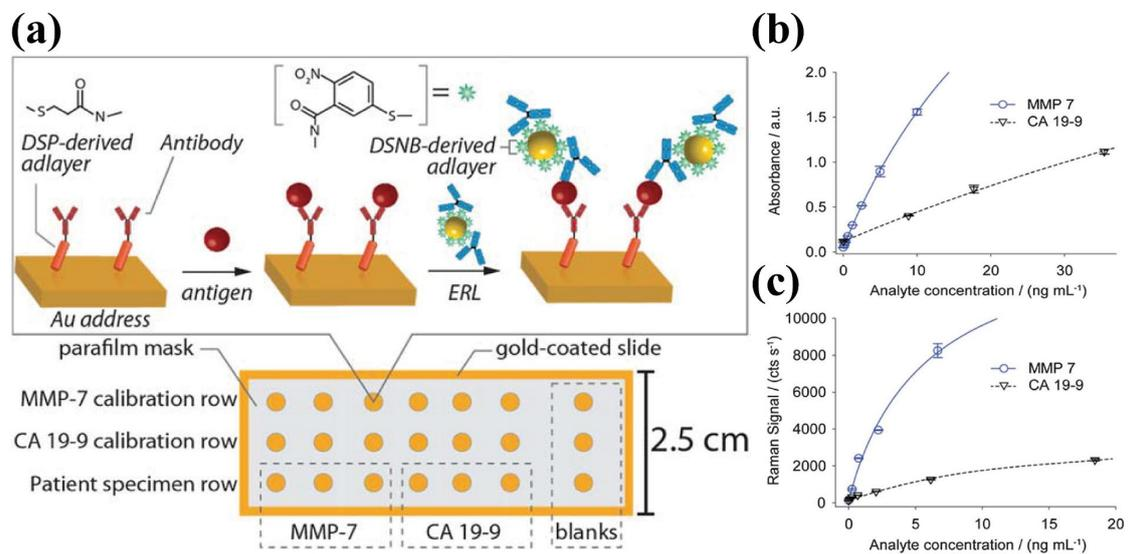
**Figure 7.** (a) Schematic of SERS array for MMP-7 and CA19-9; (b) ELISA calibration plots for the same MMP-7 and CA 19-9 standards used in (a); (c) SERS Calibration plots for MMP-7 and CA 19-9 antigen spiked into 1:4 pooled human serum: PBS buffer. Adapted and reproduced from ref. 77 with permission from the Royal Society of Chemistry.
