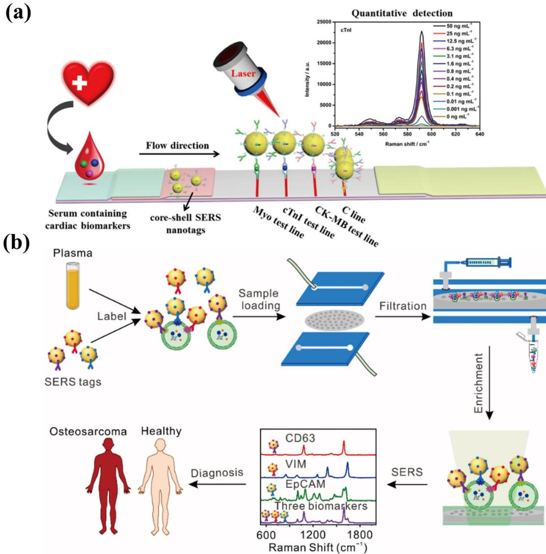
**Figure 5.** Example of integrated SERS detection platform (a) Schematic illustration of the core-shell SERS nanotag-based multiplex LFA. Adapted from ref. 45 with permission from the Elsevier Copyright 2018; (b) Schematic illustration of SERS profiling of three biomarkers on plasma-derived exosomes isolated by size-dependent microfluidic filtration for the diagnosis of osteosarcoma; adapted from ref. 46 with permission from the Elsevier Copyright 2022.
