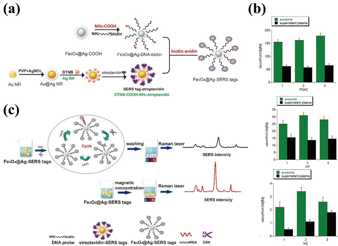
**Figure 10.** (a) The synthesis process of  $\text{Fe}_3\text{O}_4@\text{Ag}$ -SERS tags; (b) Determination of microRNA-10b concentration in exosome and residual supernatant plasma from three patients with PDAC, three normal control (NC), and three patients with CP using our SERS sensors; (c) Scheme of SERS detection of microRNA. Adapted and reproduced from ref. 79 with permission from the Elsevier Copyright 2019.
