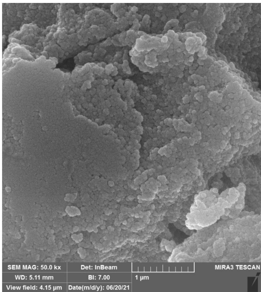
**Figure 5.** FESEM image of Silver Nanoparticles Synthesized with *polygonum aviculare L.* extract with different magnifications. Ag nanoparticles were mostly spherical., and the size was found to be between 44 and 69 nm .
