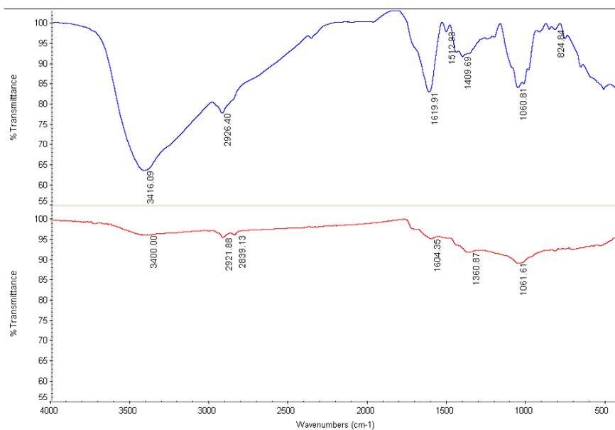
**Figure 4.** FT-IR spectrum of (a) hydroalcoholic *P. aviculare* L. extract and (b) synthesized Ag nanoparticles. As depicted, the intensity of most bands is decreased due to a decline in Ag ions.
