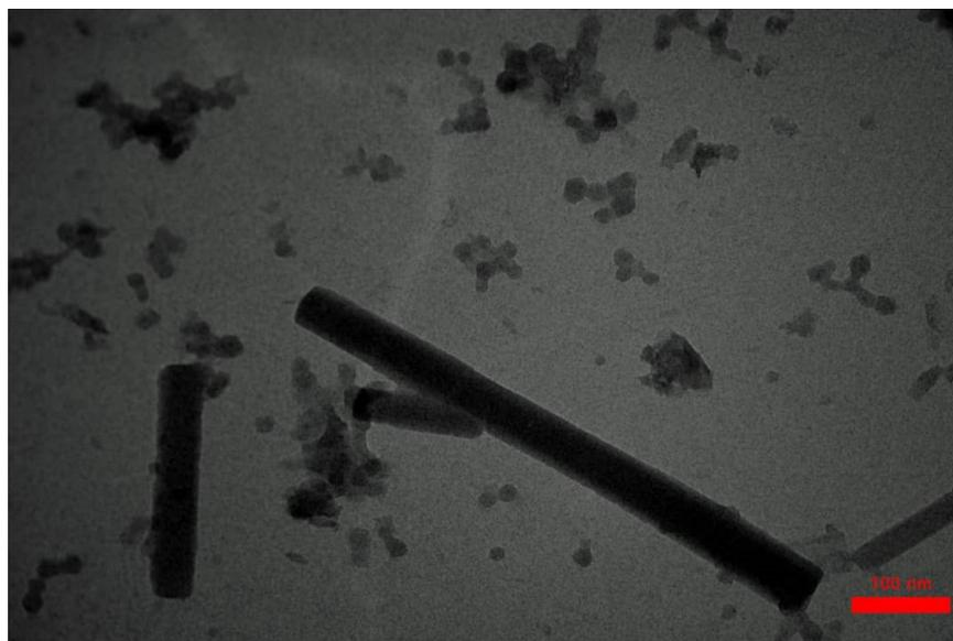
**Figure 6.** TEM image of Silver Nanoparticles Synthesized with *polygonum aviculare L.* extract. Ag nanoparticles were spherical and rod shaped.
