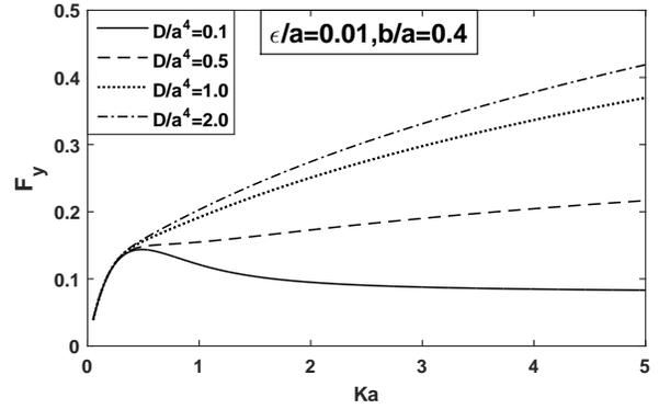
Fig.5: Magnitude of heave exciting force on prolate spheroid with fixed immersion  $f/a=2.0$
