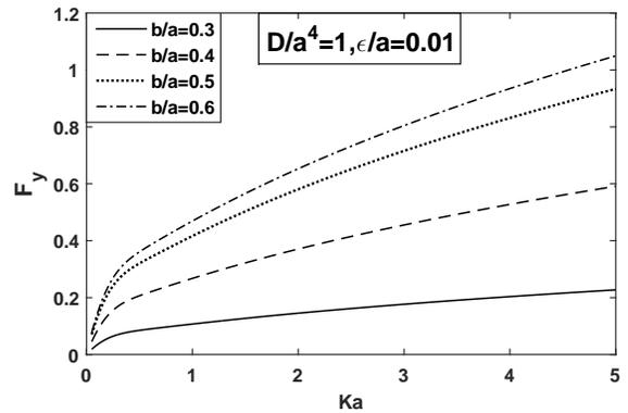
Fig.9: Magnitudes of heave exciting force on prolate spheroid with fixed immersion  $f/a=1.5$
