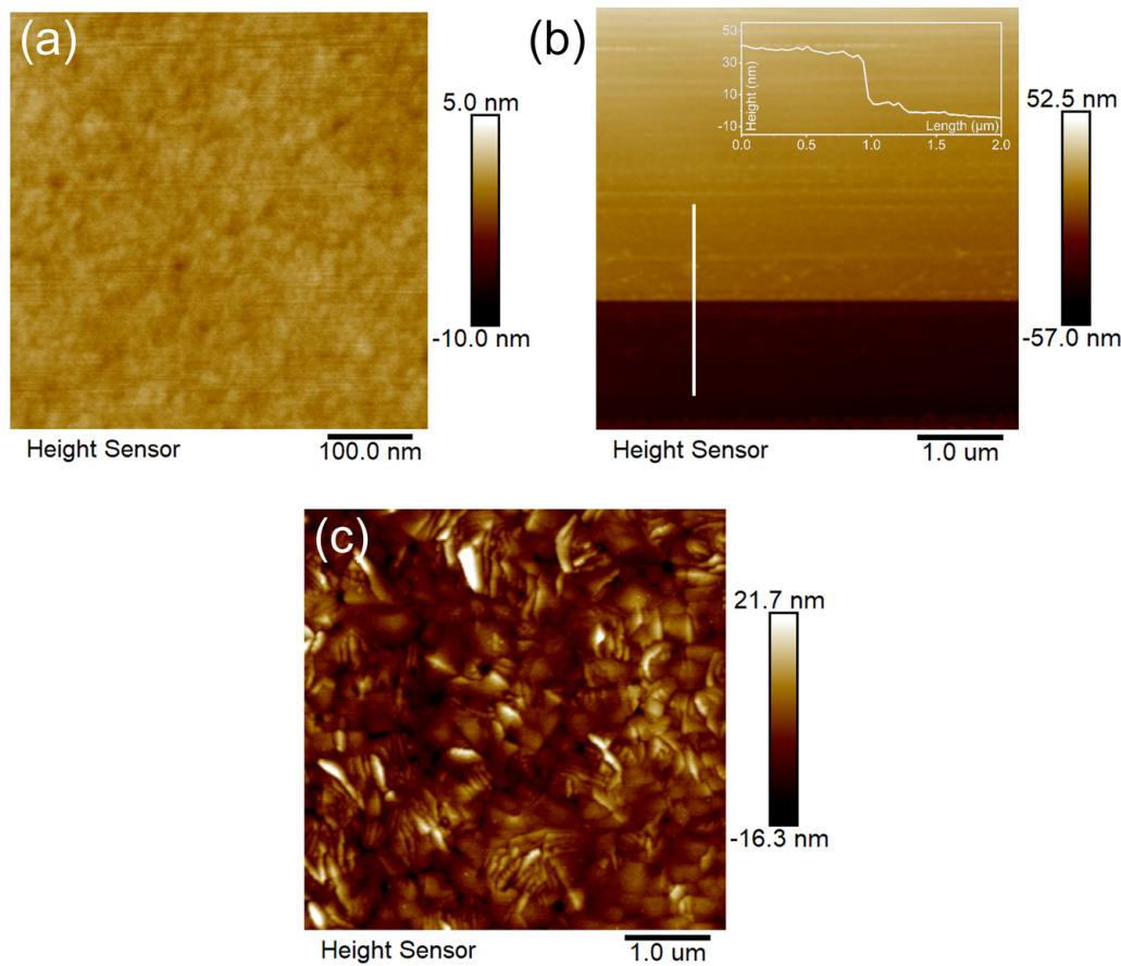
Figure 5: **Figure S5.** (a) The AFM image of the 2D  $\text{Zn}_2(\text{ZnTCPP})$  MOFs-PMMA dielectric layer. (b) The thickness measurement of 2D  $\text{Zn}_2(\text{ZnTCPP})$  MOFs-PMMA film using AFM. (c) The AFM image of the pentacene film deposited on the 2D  $\text{Zn}_2(\text{ZnTCPP})$  MOFs-PMMA dielectric layer.
