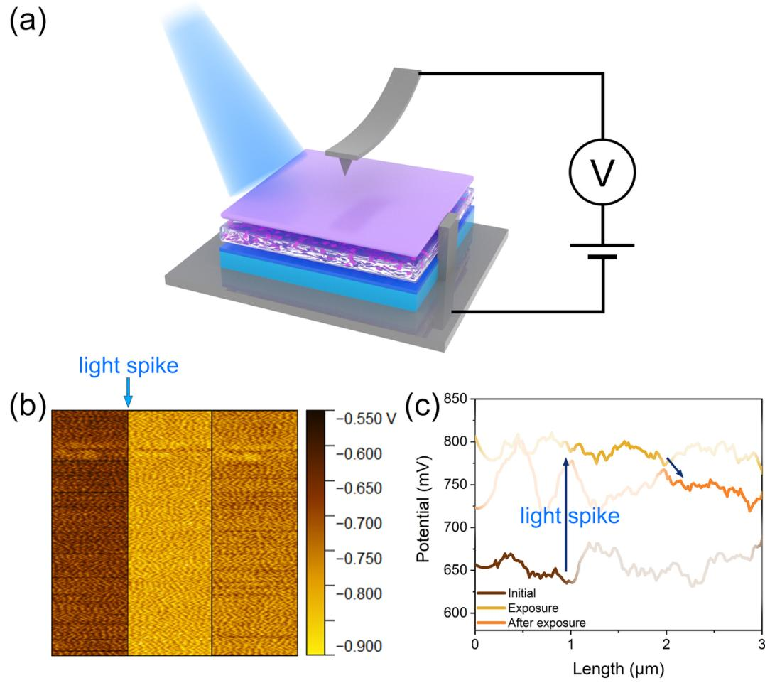
Figure 8: **Figure S8.** (a) The schematic KPFM measurement. (b) The KPFM potential image before and after the light spike. (c) The potential curves before and after the light spike.
