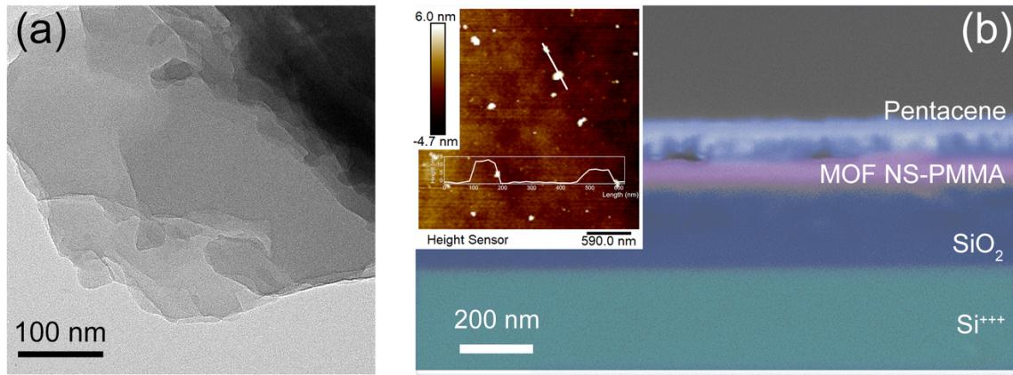
Figure 3: **Figure S3.** The characterizations of the 2D  $\text{Zn}_2(\text{ZnTCPP})$  MOFs-PMMA/Pentacene structure. (a) The TEM image of the 2D  $\text{Zn}_2(\text{ZnTCPP})$  MOFs. (b) The cross-section SEM image of the device (inset, the AFM image of the 2D  $\text{Zn}_2(\text{ZnTCPP})$  MOFs).
