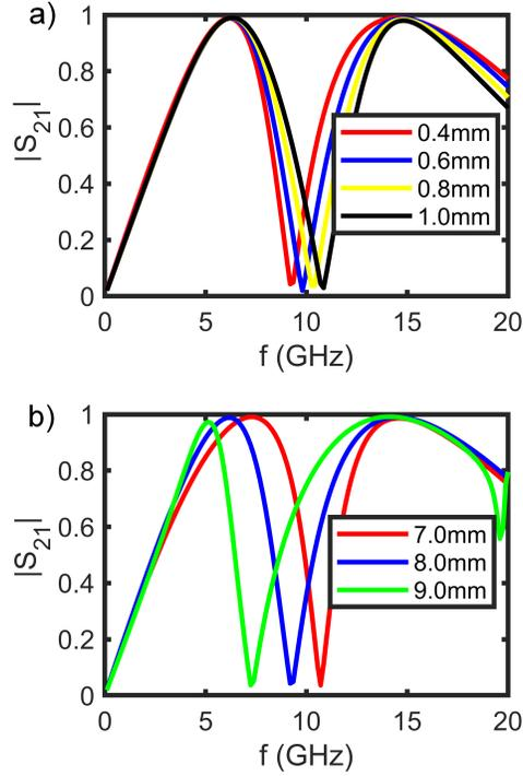
FIG. 3. Transmission spectra for different strip widths  $w_1$  (a) and lengths  $l_1$  (b) of the constituent square loop. The results have been obtained by full wave simulations. In the simulations we assumed copper as the metal, fr-4 as the dielectric substrate and a thickness of the dielectric substrate to be 0.1mm. We assumed the geometrical parameters  $D=10$ mm,  $w_2=0.1$ mm and  $w_3=2.5$ mm. In (a)  $l_1=8$ mm and in (b)  $w_1=0.4$ mm.
