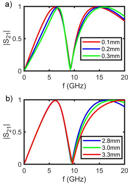
FIG. 4. Transmission spectra for different strip widths  $w_2$  (a) and slot widths  $w_3$  (b) of the constituent square slot. The results have been obtained by full wave simulations. We assumed the geometrical parameters  $D=10$ mm,  $l_1=8$ mm and  $w_1=0.4$ mm. In (a)  $w_3=2.5$ mm and in (b)  $w_2=0.1$ mm.
