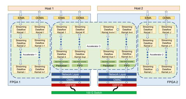
Figure 2: Three MobileNet accelerators implemented using two U280 accelerator cards
