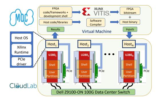
Figure 1: The Open Cloud Testbed: Hardware and software
