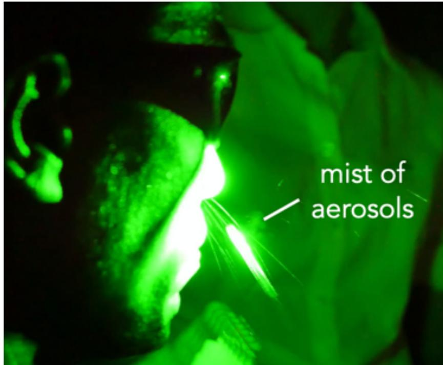
Image 1c – Most droplet production occurred with nasal expiration immediately after nasal decongestion spray
