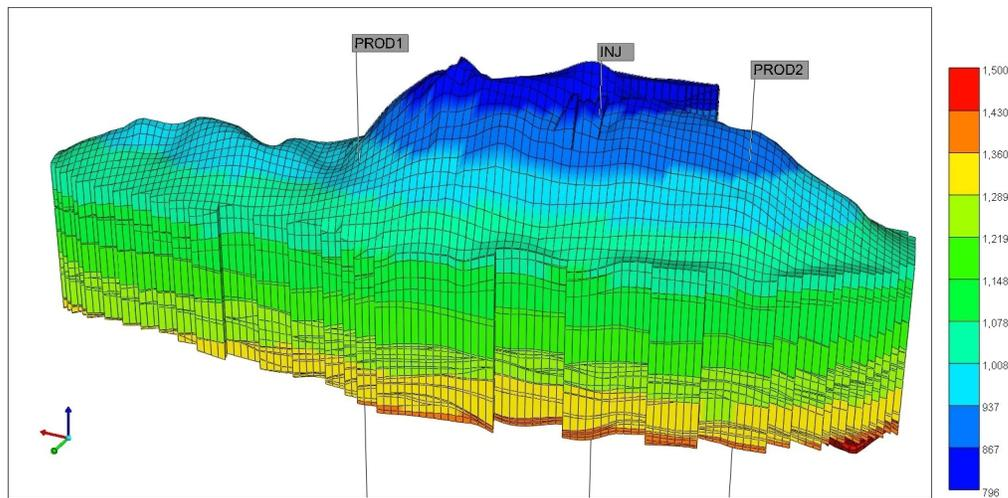
The geometry, well positions, depth and grid system of the 3D conceptual reservoir model of the selected oil field.
