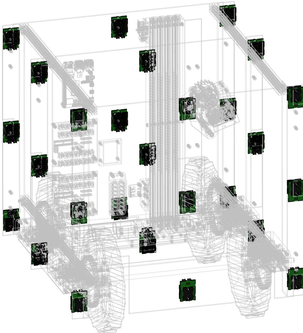
Calibration of the magnetic sensors will be done by rotating the rover on its z-axis. This will allow the rover to identify its own magnetic sources from the magnetic field of the planet or moon.
