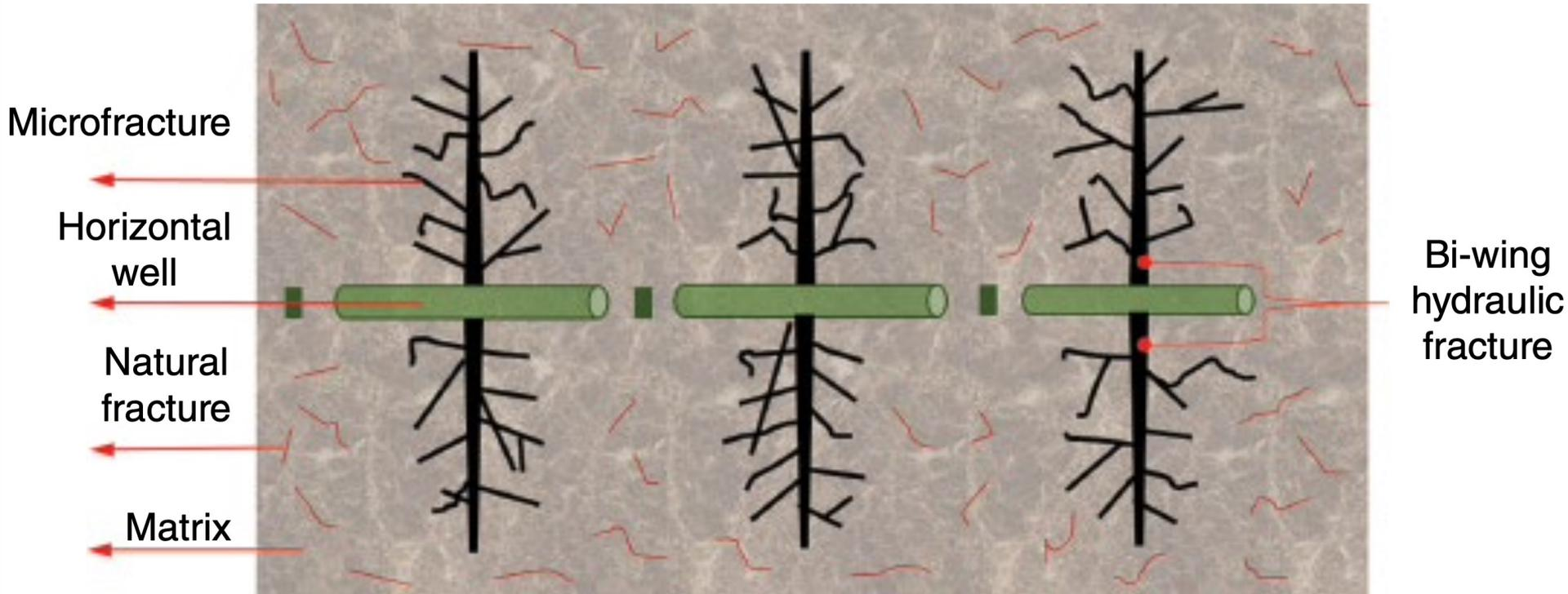
Schematic of multi-scale fracture system in the shale gas reservoir after hydraulic fracturing operations. Natural fracture, microfracture, and hydraulic fractures coexist (after Chen et al., 2019).
