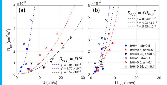
Figure 7. The relation between effective sediment-water gas transfer diffusion coefficient,  $D_{eff}$ , and (a) the time-averaged mean flow velocity,  $U$ ; (b) the time-averaged mean flow velocity within the vegetation canopy,  $U_{veg}$ , under different submergence ratios ( $U = 0.25, 0.5, \text{ and } 1$ ) and array roughness densities ( $ah = 0.1 \text{ and } 0.5$ ). Trendlines are parabolic fits to both sparse and dense conditions for each submergence ratio.
