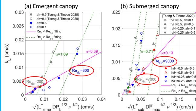
Figure 6. The linear fitting results of the emergent (left) and submerged (right) canopy fitting data by the modified SR model. The critical stem-scale Reynolds number,  $Re_{dc}$ , for the emergent case shifts from 200 on a fixed smooth bed (Tseng & Tinoco, 2000) to 300 on a sediment bed, while the critical mean flow Reynolds number,  $Re_H$ , shifts from 7000 on a fixed smooth bed (Tseng & Tinoco, 2000) to 9000 on a sediment bed.
