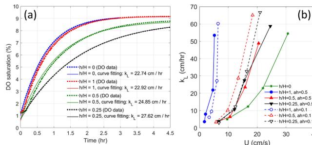
Figure 3. (a) The fittings of re-aeration process for the surface gas transfer rate,  $k_L$ , estimation. (b) The relation between surface gas transfer rate,  $k_L$ , and time-averaged mean flow velocity,  $U$ .
