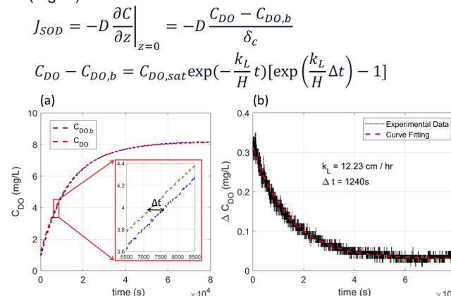
Figure 4. (a) The re-aeration curves obtained from the DO measurements near the bed (blue dashed line) and the surface (red dashed line) under flume pump frequency,  $f = 20 \text{ Hz}$ , with  $ah = 0.1$  and  $h/H = 0.25$ . (b) The fitting result of the time lag,  $\Delta t$ , based on Equation 1 and the surface gas transfer rate,  $k_L$ , under flume pump frequency,  $f = 20 \text{ Hz}$ , with  $ah = 0.1$  and  $h/H = 0.25$ .
