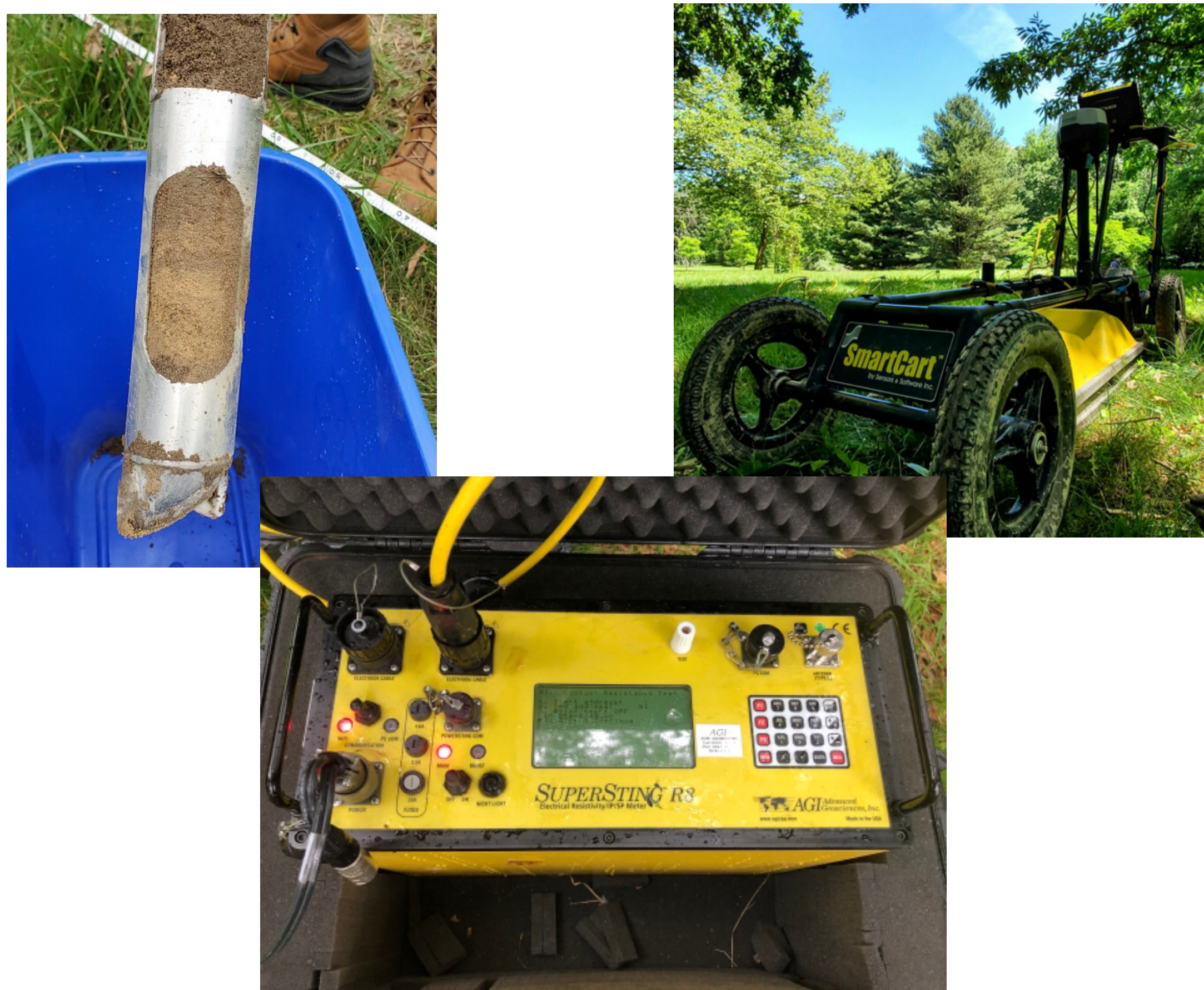
Figures 1-3. Sandy soil core, GPR mobile device, and ERT device at the Stranahan Arboretum site during data collection
