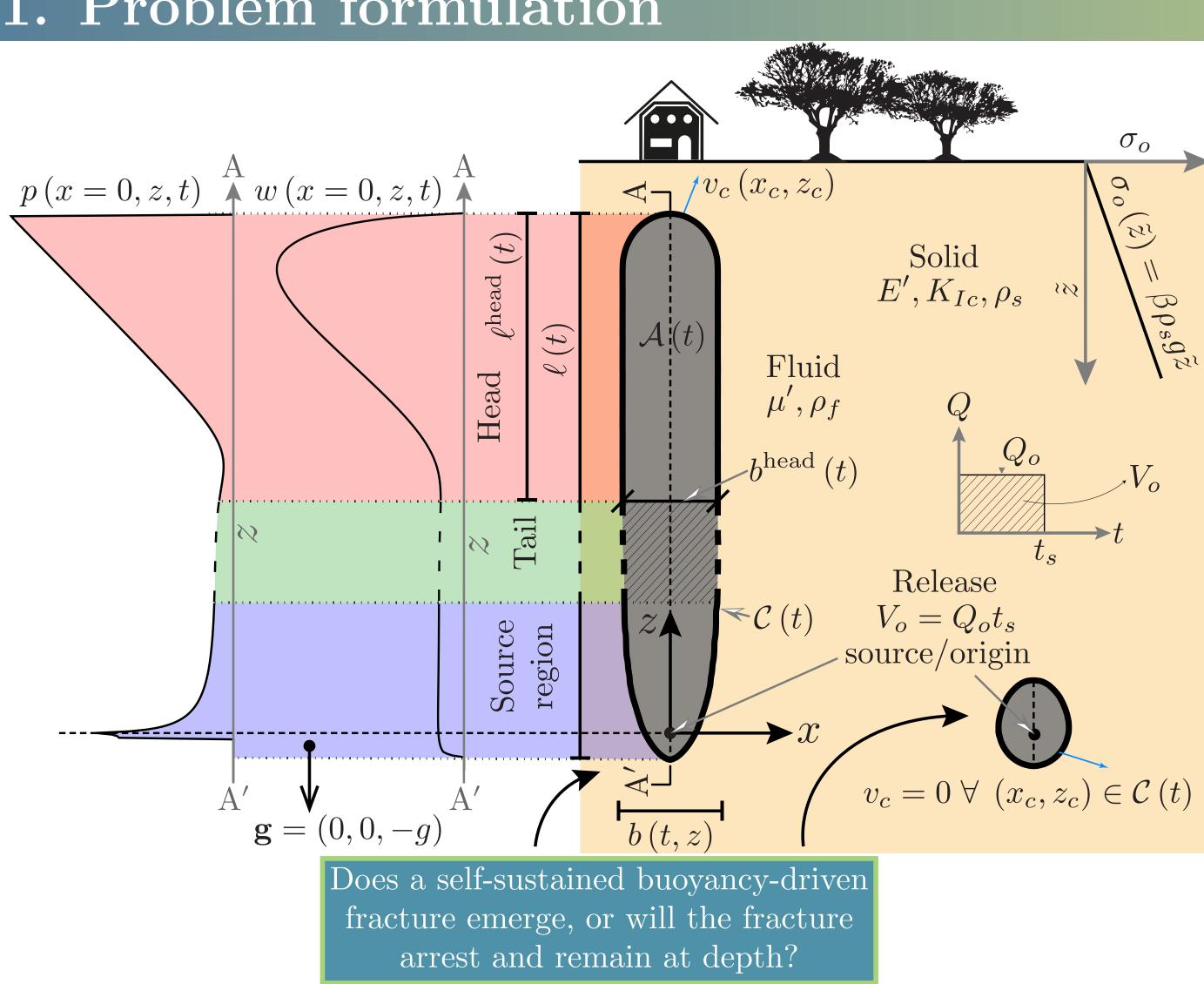
The problem of a planar mode I fracture assuming LEFM, no leak-off, and zero fluid-lag, is solved using PyFrac (Zia and Lecampion, 2020), an ILSA-based open-source solver. A scaling analysis reveals three main dimensionless coefficients
