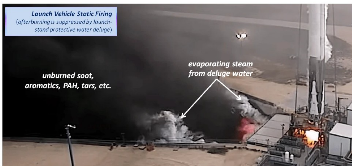
Figure 4. During static firing the deluge water below vehicle prevents facility damage to the test-stand by the hot plume, but the deluge water also quenches after-burning of the soot, aromatics, PAH, tars, etc. created by the gas generator and film coolant flows, seen as the large dark cloud (PM2.5, PAH, aromatics, etc., left). Compare this with Figure 5 post-AB shutdown (upper right). [ref. C]
