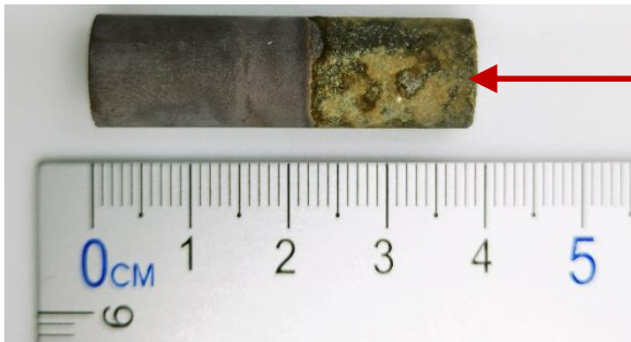
Salt deposition and severe corrosion
