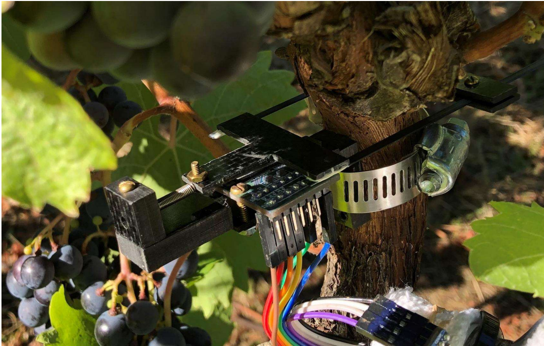
Figure 1: Dendrometer prototype installed on grapevine at Woodhall III Vineyards (Alpine, OR)
