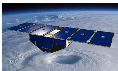
The 8 CYGNSS micro-satellites each make 4 simultaneous measurements. The standard CYGNSS data product (L1) is 1, 2, or 4 Hz measurements. Satellite motion causes the reflection point to move at 6 km/s. For coherent scattering, the spatial resolution is 1 km x 7 km (first Fresnel zone x along-track non-coherent integration assuming 1 Hz measurement rate). For diffuse scattering, the spatial resolution is ~20 km x 27 km (resolution defined by radar ambiguity function projected onto the surface).
