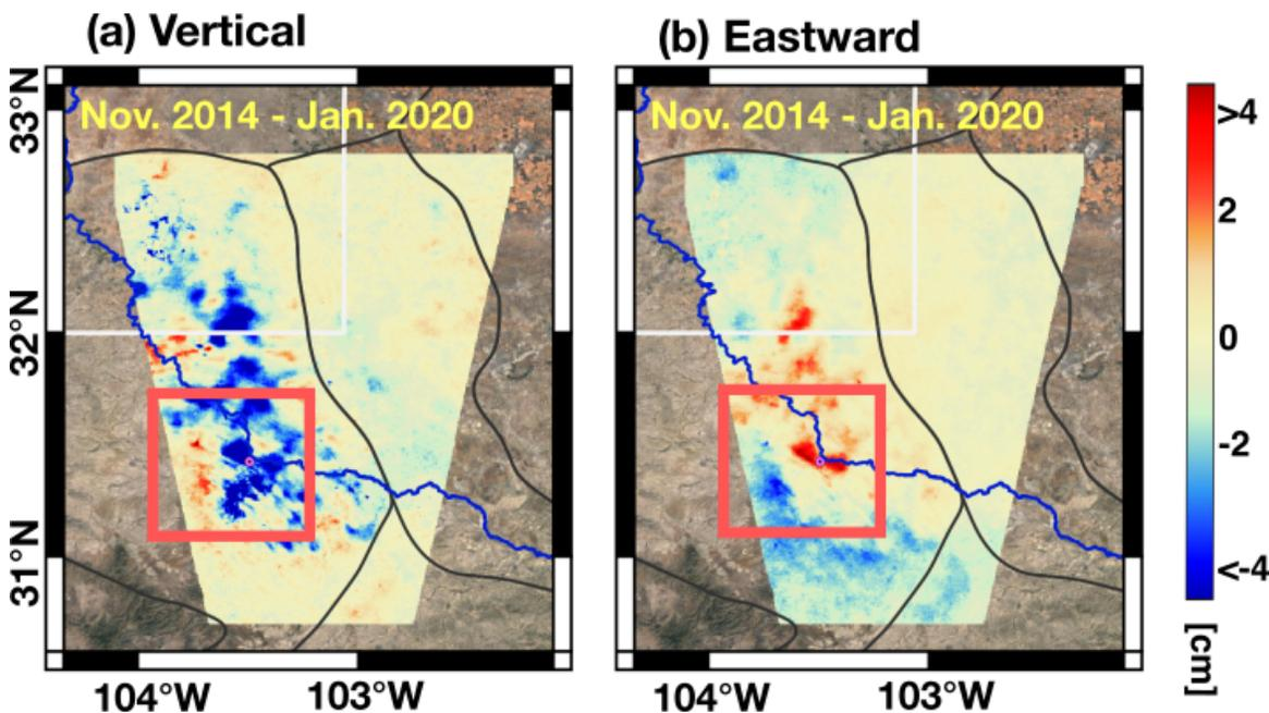
Figure 6: Cumulative vertical (left) and horizontal (right) deformation between Nov. 2014 and Jan. 2020.
