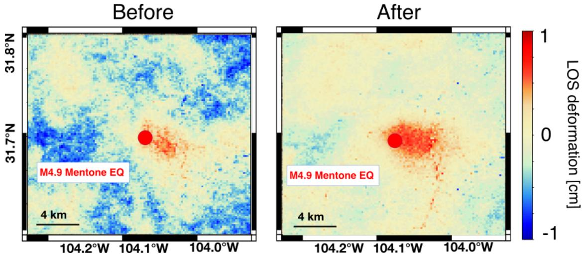
Figure 13: Coseismic stack results before (left) and after (right) detecting and removing outlier tropospheric noise dates from the average SAR interferograms.
