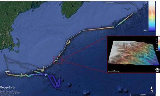
Figure 2. Bathymetric (100m resolution) rendering generated from multibeam data collected during EX1905L2 along the U.S. northwestern continental shelf edge. Inset map depicts 100m bathymetric grid generated from GMRT Synthesis of DIVE 05 site, which was absent in EX1905L2 products.
