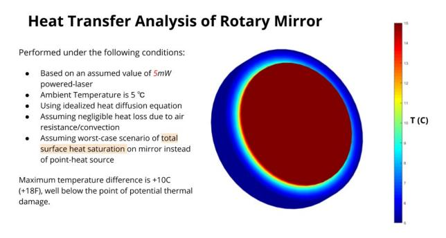
A heat transfer analysis on a rotary mirror set at 5°C was conducted as a reference point for potential spring temperatures in Northern Texas. Further analysis will be necessary with warmer temperatures for Southern Texas. Much colder temperatures will be required for Alaska but since it will be very cold the analysis probably won't be necessary.
