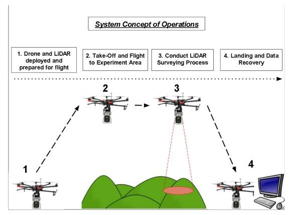
The drone, with the LiDAR attached to it, will be prepared for flight and then deployed near the target location. The drone will then fly the LiDAR over the survey area while the LiDAR fires laser pulses in a circular scan pattern. Once the survey is complete the drone will fly back to the base station and the data will be recovered from the LiDAR.
