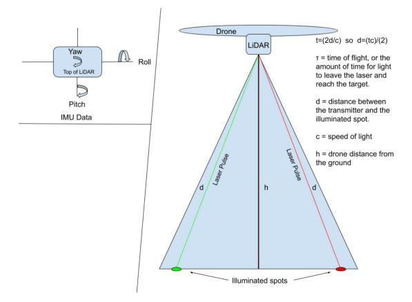
While the LiDAR is being flown over the target location it will be firing two pulsed lasers. The range equation  $d = \frac{tc}{2}$  will be used to determine the distance between the transmitter and the illuminated part of the ground where:
