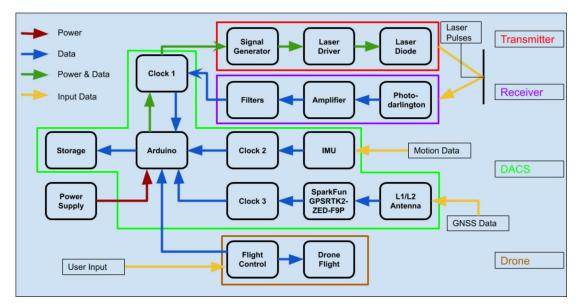
As seen in the block diagram above, the LiDAR will have three main subsystems; A Transmitter, Receiver, and DACS (Data Acquisition and Control System). Each subsystem has its own specific requirements which tie into one another.
