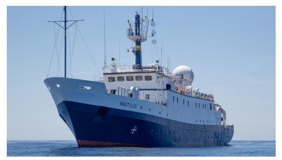
The E/V *Nautilus* is operated by the Ocean Exploration Trust and is equipped with a Kongsberg EM302 Multibeam Echosounder. Mapping data are acquired on all cruises as part of routine operations to support ROV dives and ocean exploration.
