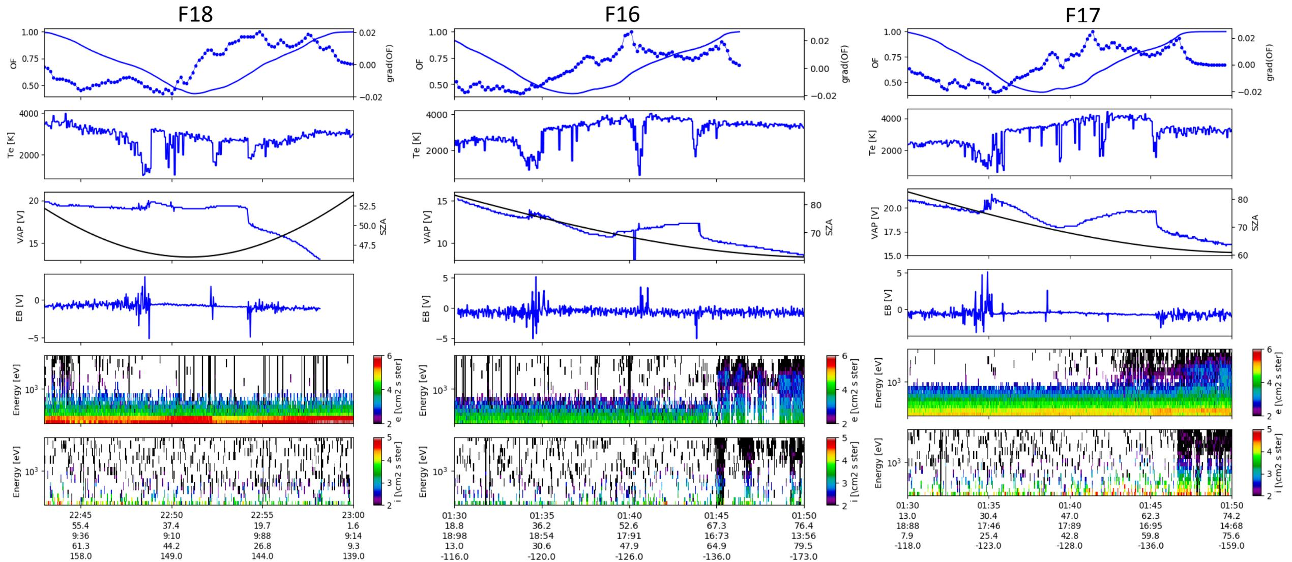
Something is affecting the ionosphere in the eclipse shadow, but our instruments are not designed to detect whatever this is directly, so we are puzzled. All three spacecraft observed similar responses as they passed through the May 2012 eclipse shadow at two different times and three different locations. With multiple sets of observations from these and other eclipses we hope to be able to track down the causes.
