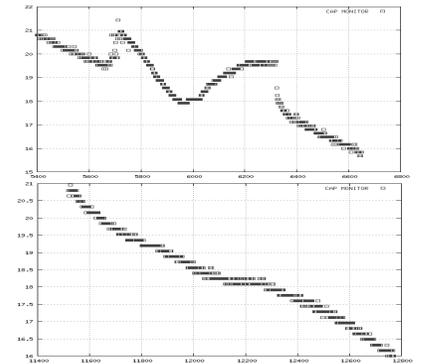
Bottom plot shows the spacecraft charges less negative (sign flipped here) as it moves northward in a nominal pass. Top plot shows an unexplained increase in negative charging in the eclipse’s shadow.
