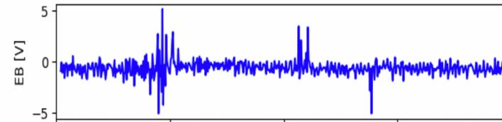
The retarding potential analyzer (RPA) samples high energy ions and electrons every two seconds and it observes high energy bursts in the regions of high EUV gradients.
