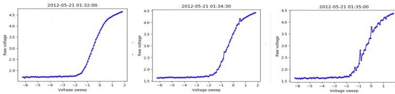
Normal smooth Langmuir probe sweep (left) gives nominal electron temperatures. The slightly noisy (center) and very noisy (right) sweeps in the EUV gradient region give the erroneous low electron temperatures.
