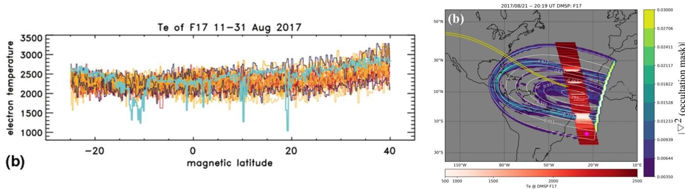
This work started with the 21 August 2017 eclipse (above) where DMSP observed strange dips in the electron temperatures at 850 km that matched the regions of large gradient in the EUV from the moon's shadow.
