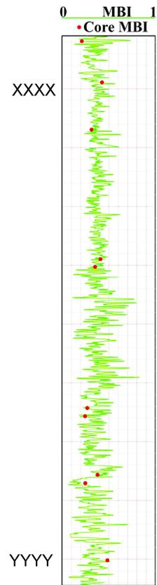
Fig. 2. A plot of continuous BI with depth estimated using Litho-Scanner log mineralogy has been shown for well-B. The data points of BI estimated from core sample mineralogical analysis have been marked with red dots.
