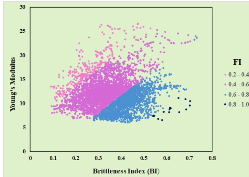
Fig.5. Cross plot of BI and E for well-B, showing the direction of increasing FI.
