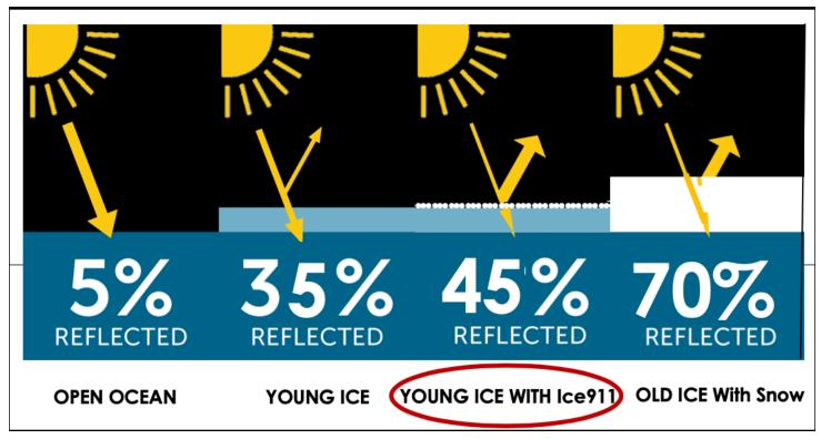
By applying a thin layer of HGM's on thin young ice, we could boost its reflectivity enough to help delay its melt, and over time, restore Arctic reflectivity. We have conducted small field tests and climate modeling studies to research and develop the method.
