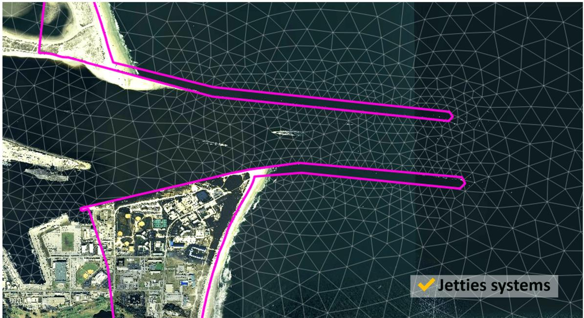
We studied the impact of the different models on tides and water surface elevations during storms.
