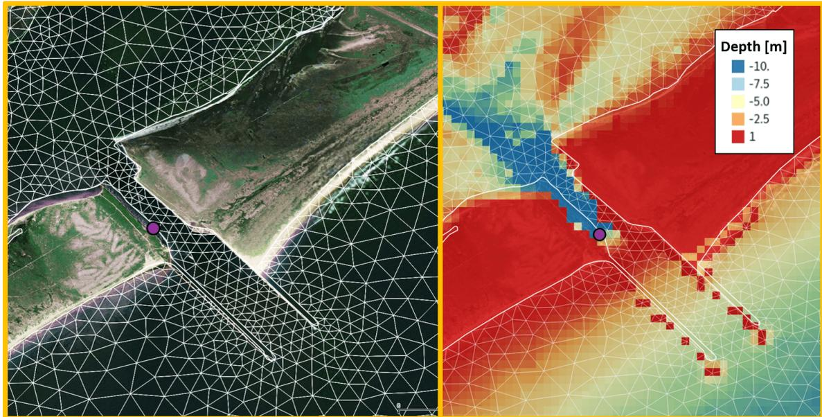
We collected ~1.5 Tb of different bathymetry datasets (see Fig. 10). We use layers of interpolation, prioritizing the newest and highest-resolution sets in areas with overlapping of information.
