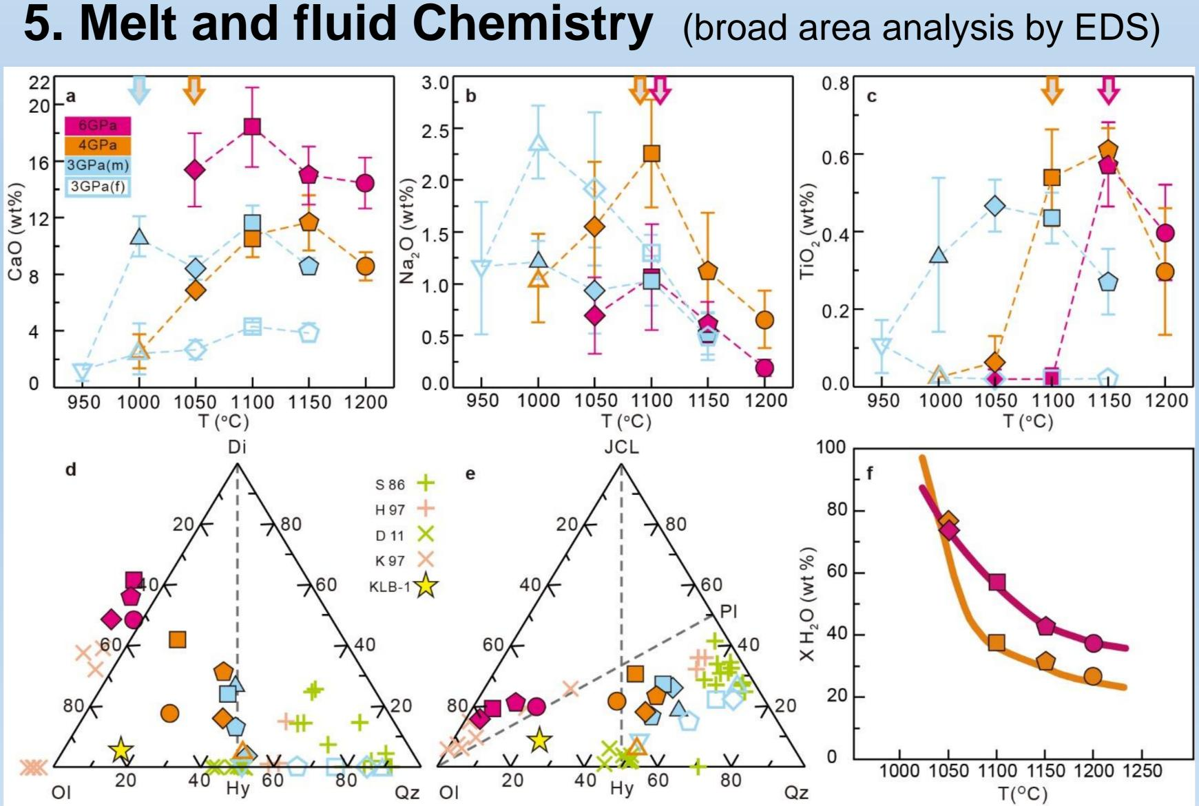
**Fluid:** Below solidus: **dacitic** at < 2 GPa, **hyperthene** at > 3 Gpa; Above solidus: dacitic to andesitic at 3 Gpa;
