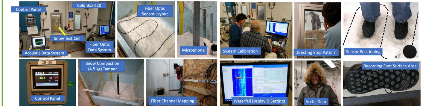
Figure 5. Snow test cell and cold box configuration set up showing control panel, fiber optic sensor layout, data acquisition system locations, snow compaction, and channel mapping.
