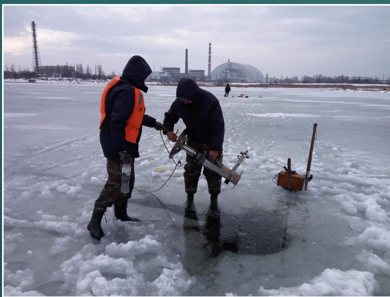
Bottom sediments core sampling at Glubokoe, Azbuchin lakes, Cooling Pond and Schekino Dam reservoir
