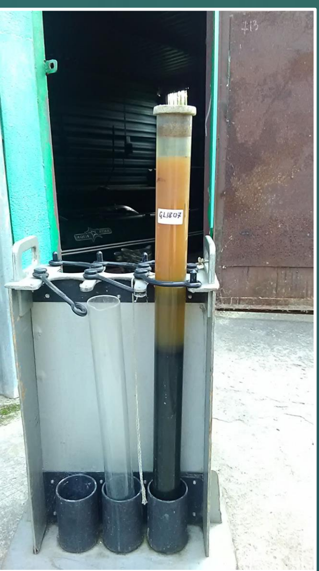
Bottom sediments core sampling at Glubokoe, Azbuchin lakes, Cooling Pond and Schekino Dam reservoir
