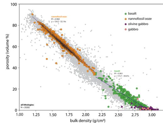
The densities are plotted versus porosity for all data (gray) and for a few selected lithologies (colored dots). Unsurprisingly, the deep crustal rocks (gabbro and olivine gabbro) have little to no porosity and high densities. Upper oceanic crust basalts and overlying sediments have fairly linear relationships between density and porosity.
