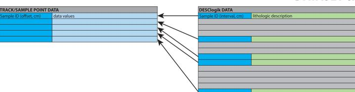
Lithologic descriptions are paired with track data based on the Expedition, Site, Hole, Core Type, Core, Section, and point (track and sample measurements) or interval (cm range) within the section.
