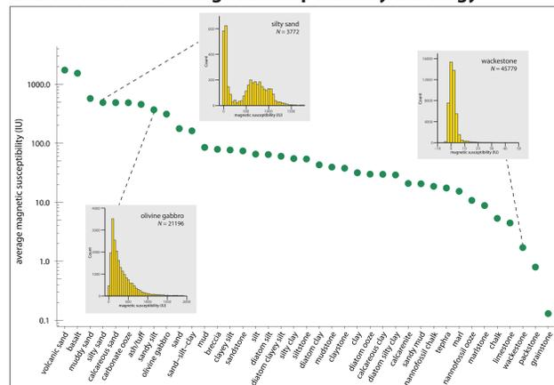
The magnetic susceptibility values for whole-round core sections measured on WRMSL are plotted versus the primary lithology. Note the large number of observations per lithology relative to the MAD density shown above. Uncertainties are not shown because they would be skewed on the log plot and because the distributions of susceptibilities for some lithologies can be multi-modal, as shown in the histograms.
