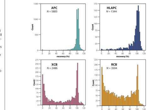
Recovery by coring type. APC = advanced piston corer. HLAPC = half-length advanced piston corer. XCB = extended core barrel. RCB = rotary core barrel. Recovery greater than 120% not included; may be the result of fall-in rather than recovery. Expeditions include only those in the table. A more extensive investigation of the success of the coring systems is being done by H. Evans and B. Clement (2019, in progress).
