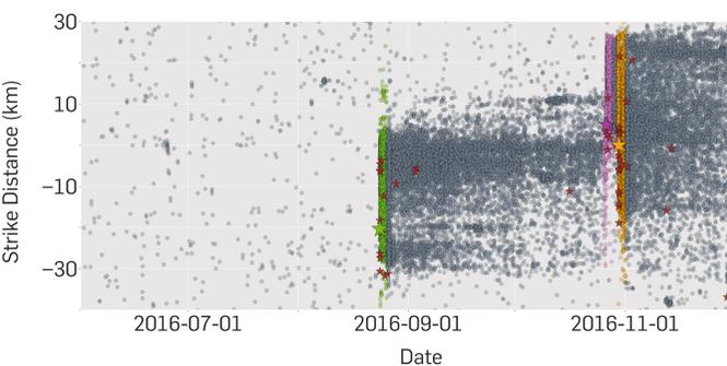
Figure 2: Earthquake occurrence along strike (Norcia mainshock at position zero). Brown stars denote earthquakes with  $M \geq 4$ . The standard catalog from INGV is used before the Amatrice mainshock. Afterwards, the catalogs from Chiaraluce (2017) and Improta (2019) are combined. Colored earthquakes denote the early aftershock sequences of each mainshock.
