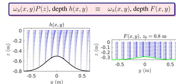
Figure 2: Vertical velocity profile for  $z_0/H = 0.8$ . Left: Flow with vertical structure  $P(z)$  and depth  $h(x, y)$ . Right: Uniform flow with depth  $F(x, y)$ . The surface flow in both cases is exactly the same.
