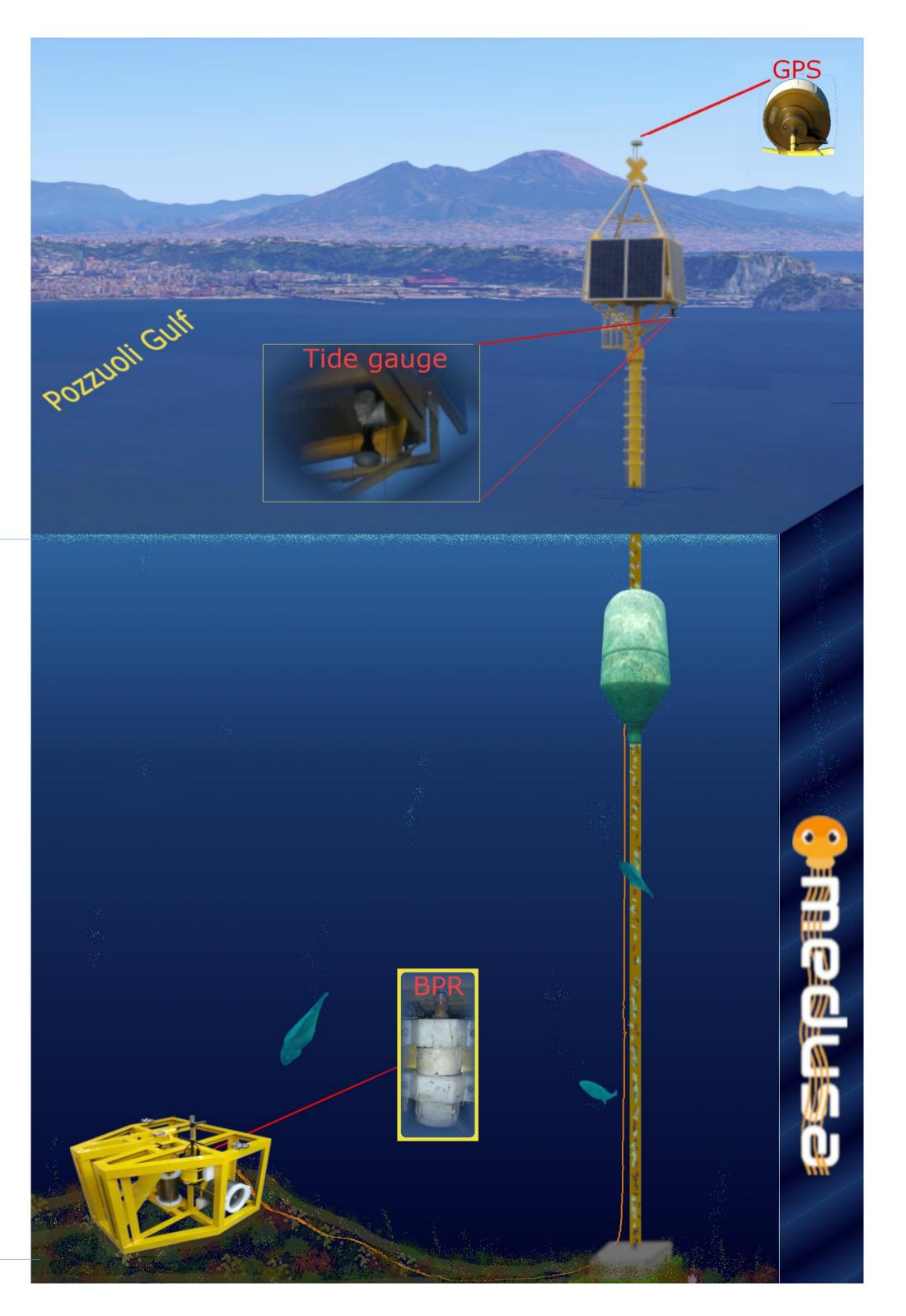
Each seafloor module includes the geophysical and oceanographic sensors; in particular, a three-component broadband seismometer (Trillium) a low-frequency hydrophone and an BPR (Paroscientific 8CDP-130I). A single-point, three-component, water-current meter and a water-temperature sensor were also installed on the C buoy module to monitor the marine environment. Status and control sensors are also presents in the module.
