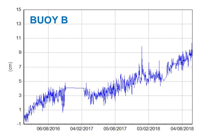
GPS data are acquired at 30 s sampling intervals and processed in kinematic mode. The reference station chosen to process the GPS seafloor data is the LICO station (see previous map), located outside the Campi Flegrei caldera, at a distance of about 10 km from the caldera center
