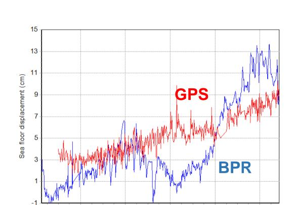
Comparison of the sea floor displacement measured by the BPR and GPS. The BPR displacement has been obtained as difference of time-series C – D (see previous figures). The trend of the two measures is consistent. A
