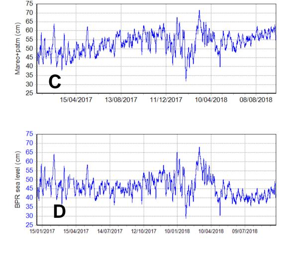
Seal level recorded by the Naples mareograph adjusted by the changes in barometric pressure (inverted barometer effect)
