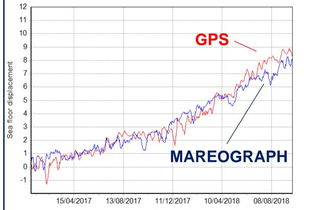
Seafloor vertical displacement measured by C buoy mareograph (blu line) is computed by the difference between the data of the time-series of two previous figures (A - B).
