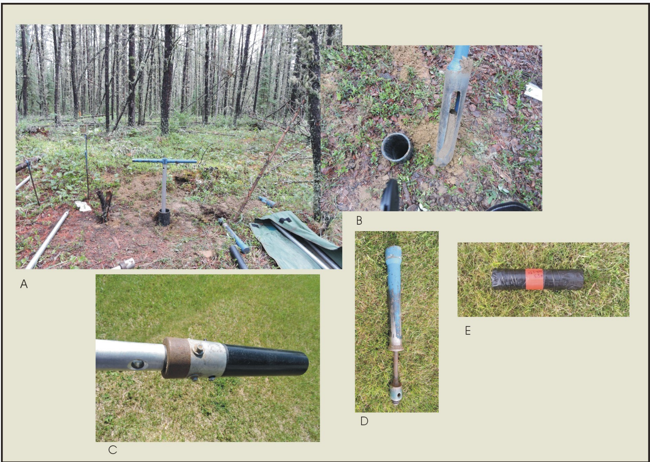
Figure 6 Luminescence dating sample extraction using auger. Desired depth is reached by extracting successive tailings retained in drill bit (A-B). Opaque sampling module is then attached to end of drill stem (C) and hammered downwards using a slide hammer (D). Extracted sample is packaged to shield from sunlight (E).
