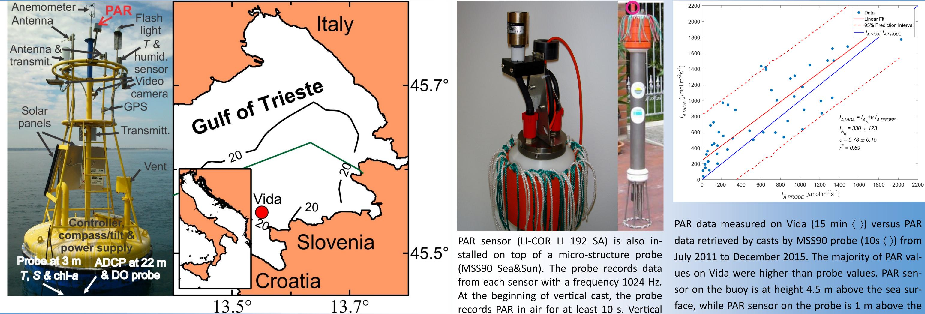
The coastal buoy Vida is located in the northernmost part of the Adriatic Sea, the Gulf of Trieste. PAR sensor on buoy Vida (LI-COR LI 190 SL 50) is mounted at the height 4.5 m. PAR data are streaming with a frequency 4.26 Hz to the land receiving station 3.7 km away.
